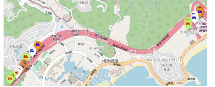
Figure 8: Mesoscopic (driver-trip) level illustration. Detection of car abnormally slowing using CAD3 (green), AD3 (white), and centralized (orange). Given the car is moving southwest to northeast, the red car icon corresponds to driving behavior being detected as abnormal, and a blue icon as normal. Only CAD3 detects abnormal driving accurately and stably, while AD3 still fluctuates, and centralized remains unpredictable.
