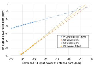
Fig. 8. Linearity measurement of array receiver to main beam direction.
