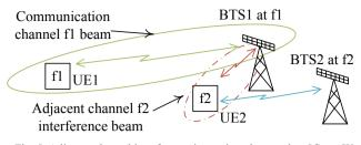
Fig. 5. Adjacent channel interference in receiver due to other 5G mmW band transmission.
