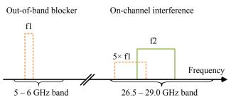
Fig. 2. Wi-Fi/LTE LAA band interference scenarios to 5G mmW band.
