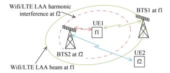
Fig. 1. Wi-Fi/LTE LAA harmonic interference scenario to 5G mmW.
