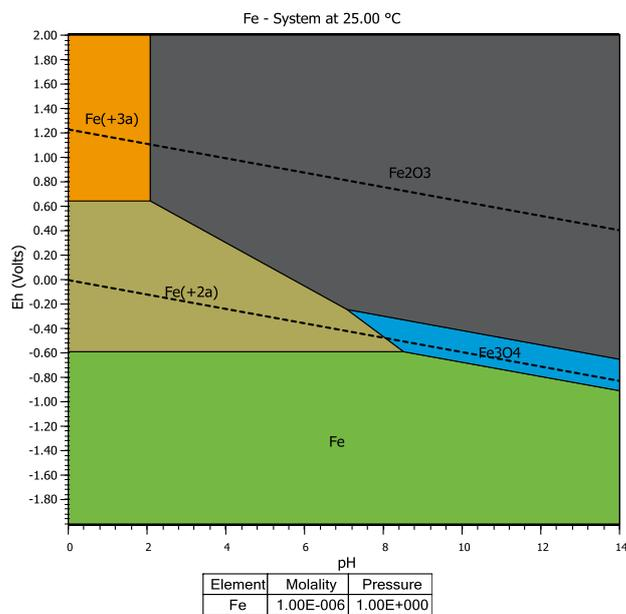
Fig. 12. Pourbaix diagram drawn with the EpH module of the HSC Chemistry.
