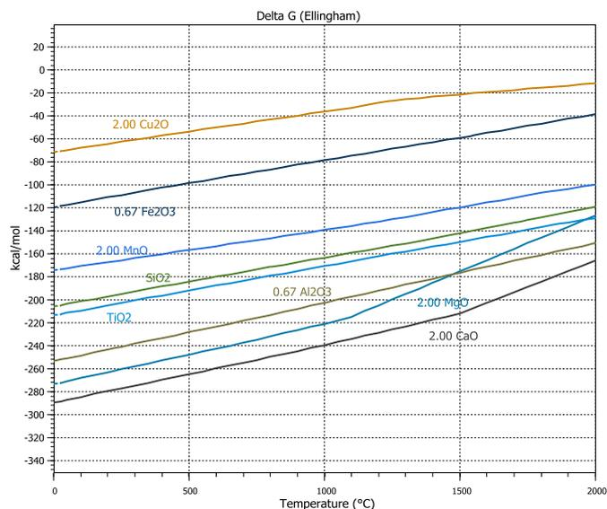
Fig. 10. Ellingham diagram drawn with the Dia module of the HSC Chemistry.
