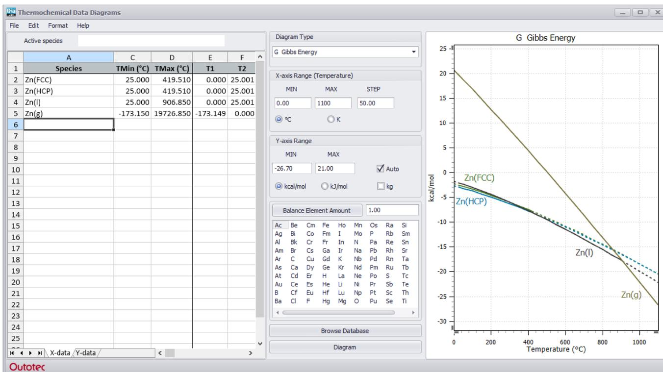
Fig. 4. Use of the Dia module of the HSC Chemistry to illustrate the Gibbs free energies of different states of zinc as a function of temperature. The phase with the lowest value of Gibbs free energy is the most stable in each temperature.
