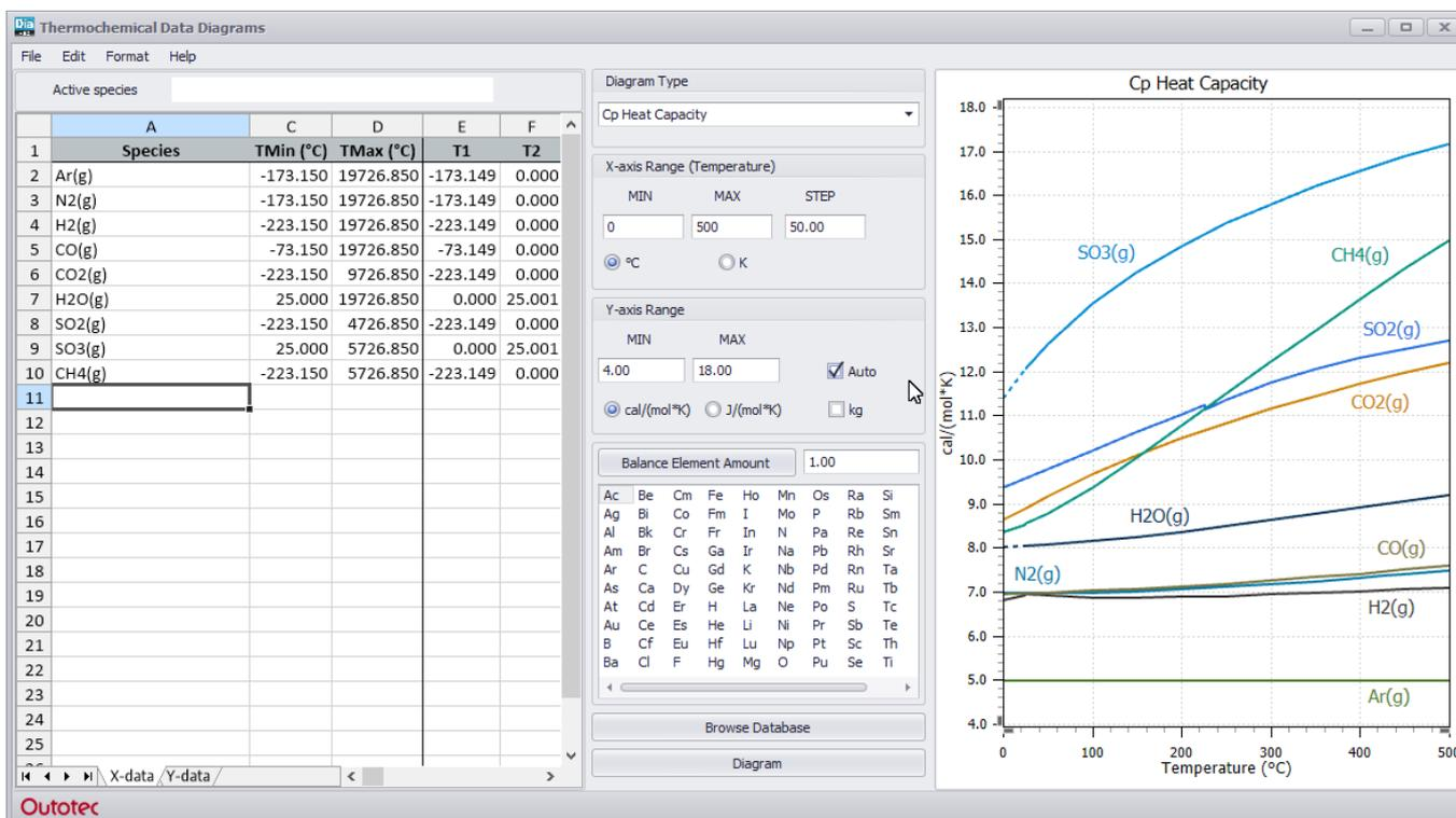
Fig. 5. Use of the Dia module of the HSC Chemistry to illustrate the change of heat capacities as a function of temperature for selected gas components. The figure illustrates how the values of heat capacity are increased with the increasing complexity of the gas molecules.
