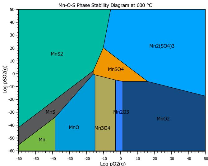
Fig. 11. Kellogg diagram drawn with the Lpp module of the HSC Chemistry.
