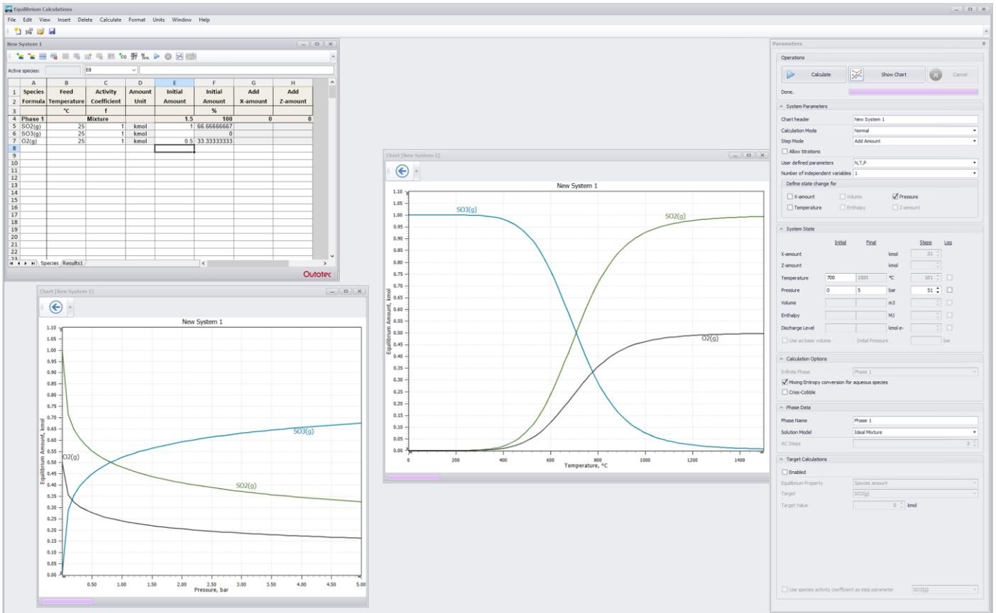
Fig. 2. Example on the use of the Gem module in HSC Chemistry. This example illustrates the Le Chatelier's principle by showing the effects of temperature and pressure on the chemical equilibrium between sulphur dioxide (SO<sub>2</sub>) and sulphur trioxide (SO<sub>3</sub>).
