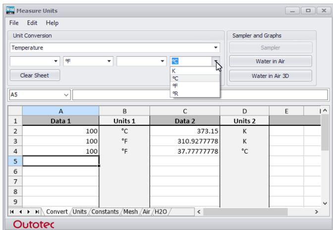
Fig. 9. Example of unit conversions using the Mea module in the HSC Chemistry.
