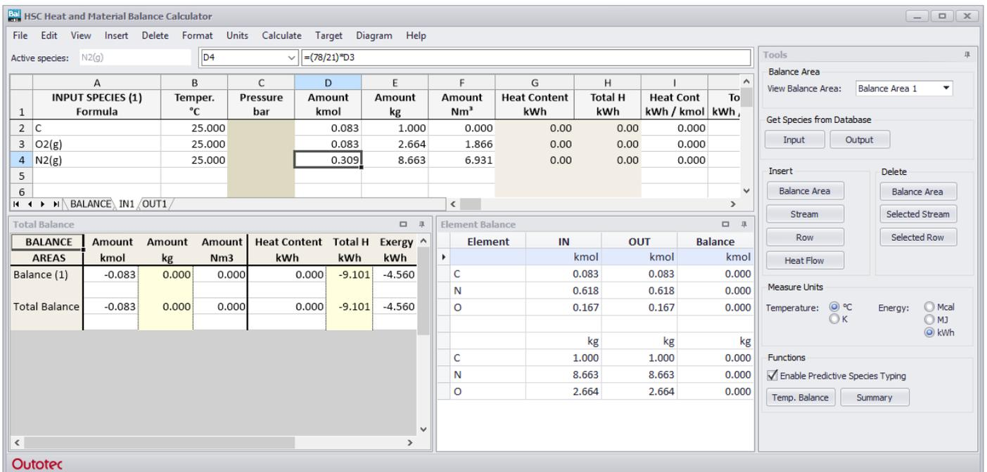
Fig. 3. Example on the use of the Bal module in HSC Chemistry. This example illustrates how much heat is released when burning carbon with air.
