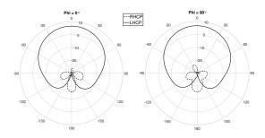
Fig. 3. LHCP Co-pol vs Cross-pol radiation pattern
