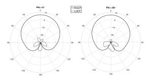
Fig. 2. RHCP Co-pol vs Cross-pol radiation pattern
