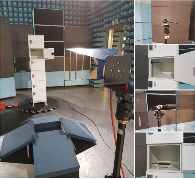
Fig. 6: A photograph of the radiation pattern measurement setup in an anechoic chamber and measured antenna placements.
