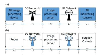
Fig. 6: (a) Latency breakdown for use case II-A (b) Latency breakdown for use case II-B
