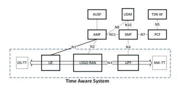
Fig. 3: The proposed network architecture.
