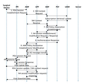
Fig. 1: The message flow diagram for device registration.
