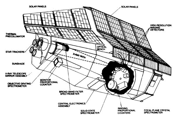
FIG. 16. Schematic representation of the *Einstein X-ray Observatory*. From Giacconi et al., 1979.
