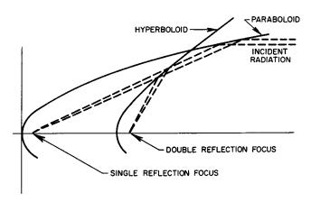
FIG. 13. Principle of x-ray grazing incidence telescope. Illustration of R. Giacconi.
