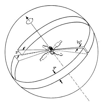
FIG. 3. The fields of view of the detectors on the *UHURU* satellite. From Gursky, 1970. Reprinted in Giacconi and Gursky, 1974, p. 95.
