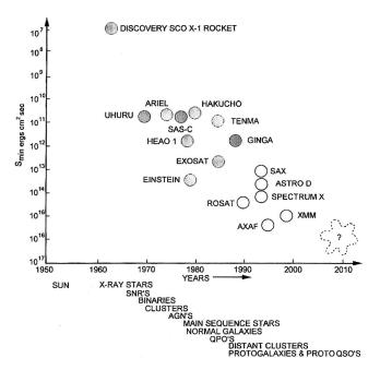
FIG. 21. The sensitivity achieved by various x-ray missions (1970 to 2000). Illustration of R. Giacconi.
