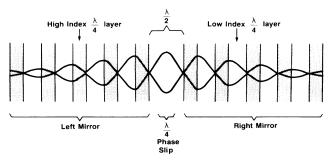
FIG. 1. A Fabry-Perot resonator made of multilayer dielectric mirrors with a space of one-half wavelength between the left and right mirrors. The net effect is to introduce  $\lambda/4$  phase slip in the overall periodic structure.
