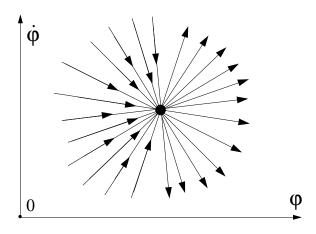
Figure 4: If **A** had the eigenvalues  $\lambda_1 = \lambda_2$ , then the singular point  $\Psi_c^+$  would be a nodal point and there would be a continuous set of trajectories passing through it. To illustrate this we plot here the phase curves in the particular case of a degenerate nodal point. The form of the equation of motion (II.13) excludes such types of singular points and therefore prevents the possibility of such transitions.
