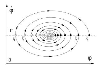
Figure 3: Phase curves in the neighborhood of the singular point  $\Psi_c^+$  are plotted for the case of the pure imaginary  $\lambda$ . Here we assume that the singular point is a focus.
