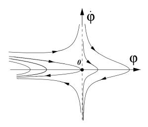
Figure 6: The typical behavior of the phase curves in the neighborhood of the critical line where  $K(\varphi) = 0$  (here  $\dot{\varphi}$  axis ) is plotted for the case when  $K'_c > 0$ ,  $V'_c = 0$ , and  $V''_c > 0$ .
