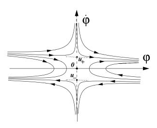
Figure 5: The typical behavior of the phase curves in the neighborhood of the critical line where  $K(\varphi) = 0$  (here  $\dot{\varphi}$  axis) is plotted for the case when  $K'_c > 0$  and  $V'_c < 0$ . Horizontal dashed lines are the analytically obtained separatrices  $\dot{\varphi}_{\pm}$  and  $(0, u_{\pm})$  are the points of transition.
