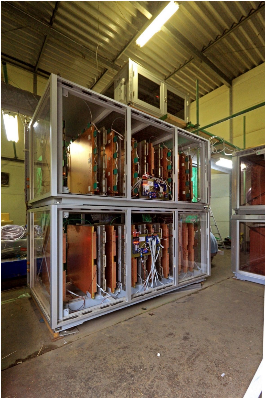
Fig. 2. Photograph of three Multi-Wire-Proportional-Chamber-based Muography Observation System (MMOS) [40]. Eleven MMOS operated in the Sakurajima Muography Observatory during 2021. The MMOS cover a surface of 8.25 m 2 .
