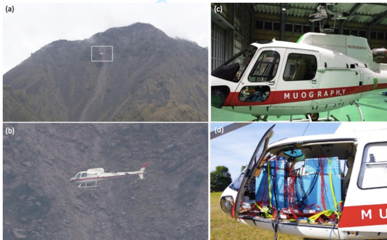
Fig. 1. Airborne muography observations at Unzen volcano, Japan [39]. a) Panoramic view of the volcano with the position of the helicopter carrying the instrument, the white rectangle indicates the position of the helicopter; b) blow-up image of the helicopter seen in panel a; c) helicopter without instrument; d) helicopter loaded with the instrument.
