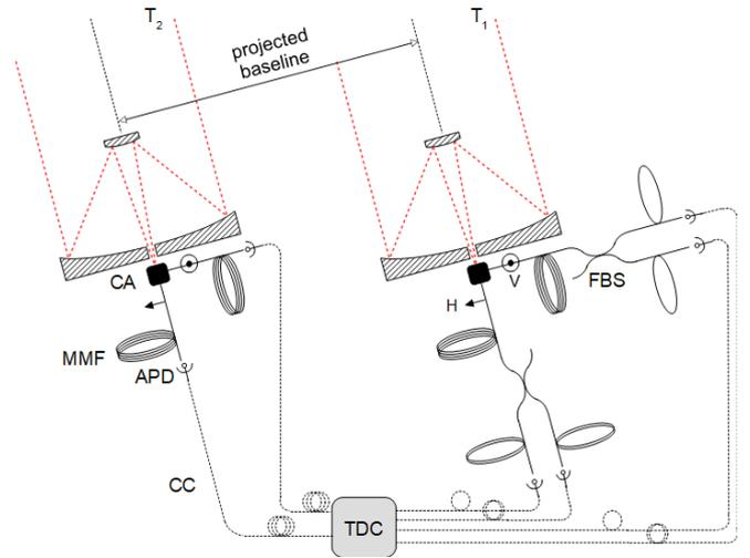
**Figure 1.** Experimental setup to measure the spatial intensity correlation function on two orthogonal polarizations (labelled H for horizontal and V for vertical).  $T_1$  and  $T_2$ : telescopes, CA: coupling assembly, see Fig. 2 for more details, MMF: multimode fiber, FBS: fibered beamsplitter, APD: avalanche photodiode, CC: 50  $\Omega$  coaxial cables, TDC: time-to-digital converter.
