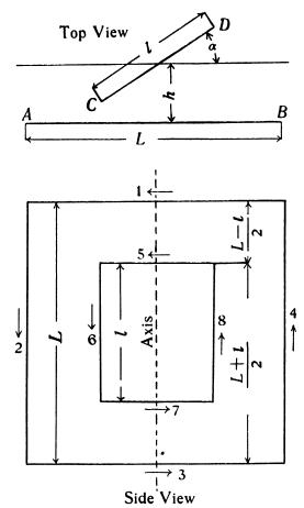
Turning our attention to the horizontal segments, let us measure x'and y' along segments 1 and 5, respectively, from their midpoints and positive in the direction of the arrow; it is then seen from the figure that the distance  $r_{15}$  between the two corresponding points is given by
