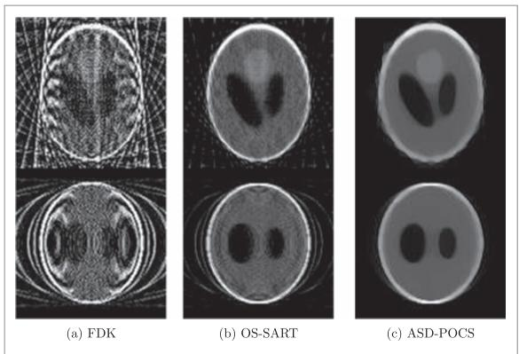
**Figure 6.** Cross-section of the image reconstructed from data from 20 projections of the 3D Shepp–Logan phantom. While an extreme case, the increased performance of the minimization algorithms over FDK is evident, especially for ASD-POCS. Times for this limited-projection example are all below a minute.
