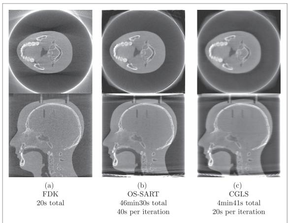
**Figure 5.** Cross-section of the image reconstructed from data from the RANDO head phantom by three different algorithms. FDK has noise across the entire image and significant strike artefacts (see top image). OS-SART and CGLS create a smoother image, removing most artefacts and having a clearer separation between tissues.
