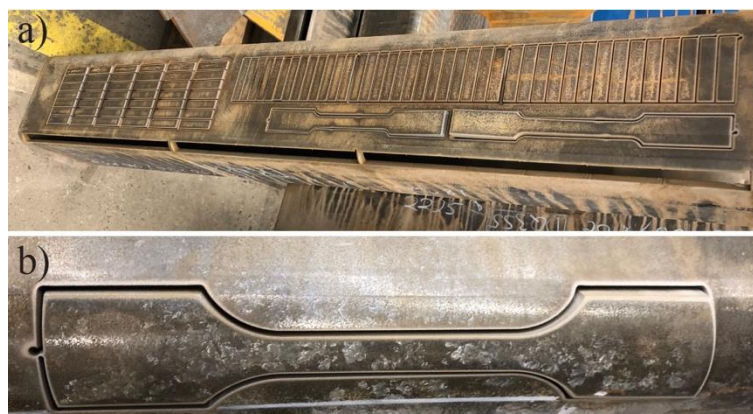
Figure 2. Examples of water-cut Charpy-V impact toughness and tensile test samples from a) flat side and b) corner of rectangular hollow section.
