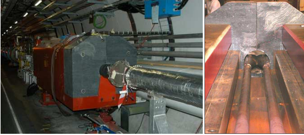
Figure 1.3: Photo of the TAN absorber located 140 m from the IP. Left: TAN fully assembled in the LHC tunnel seen from the IP side. Right: TAN during assembly at CERN seen from the top facing the IP. The 96 mm gap between the two beam pipes allows space for installation of detectors.
