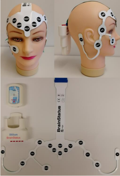
Fig. 1. EEG electrode set and device used for data collection
