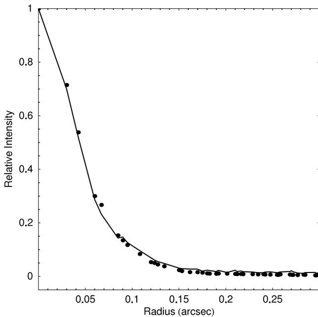
FIG. 2.—PSF derived from stars in the image shown at two positions: near the center of the image (line) and near the edge of the image (circles).
