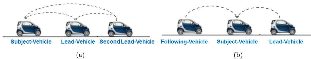
Figure 1. a) Platoon scenario presented in [39] and b) platoon scenario presented in [40]. Grey arrows indicate the communication links carrying data among vehicles
