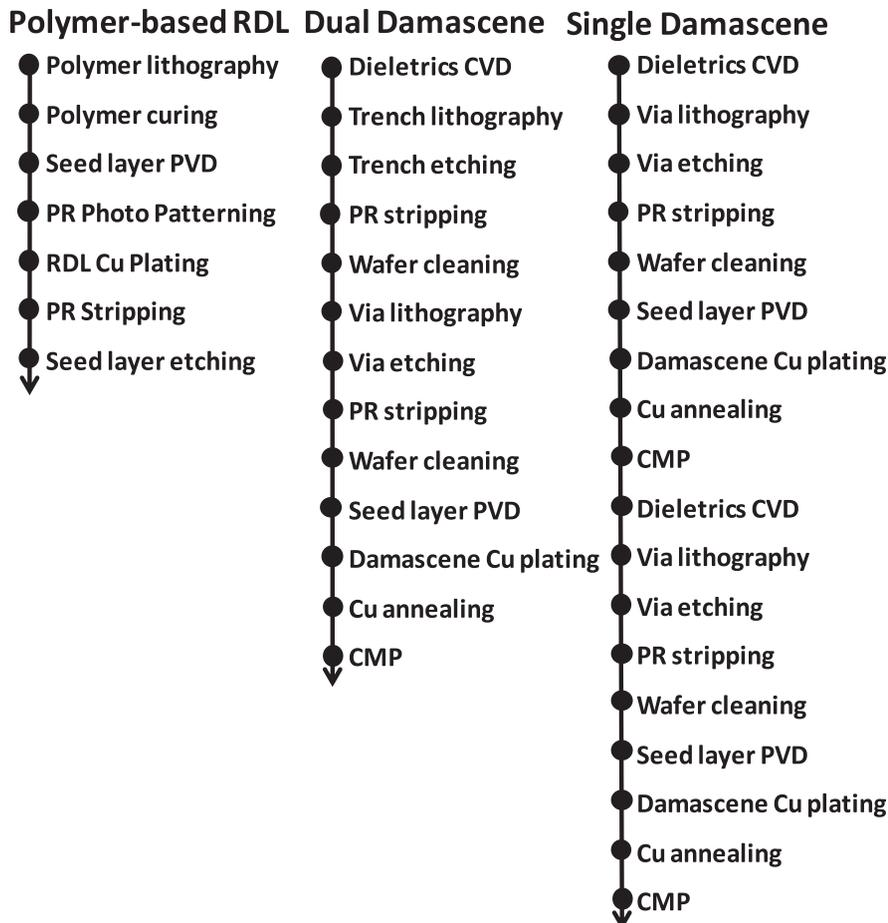
FIG. 18. Comparison of process steps of different Cu wiring processes, i.e., polymer-based RDL, dual damascene, and single damascene.
