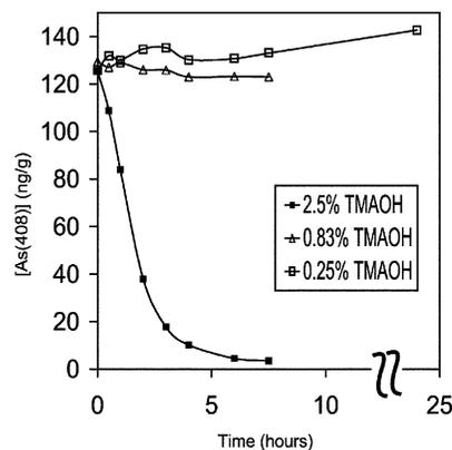
**Fig. 4** Degradation of As(408) at 60 °C in time using three different concentrations of TMAOH.
