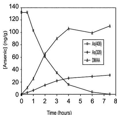
**Fig. 5** Degradation of As(408) and formation of As(328) and DMAA in 253 mM NaOH at 60 °C.
