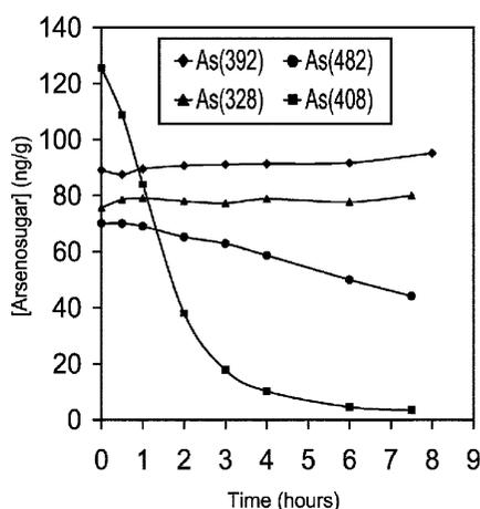
**Fig. 2** Degradation of four arsenosugars in 2.5% tetramethylammonium hydroxide (TMAOH) at 60 °C.
