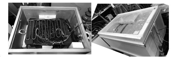
Figure 2 - Climate control units. Left: Position of the freezing coil and (right) the final set-up of the units covered with insulation material (Photos: Elisangela Heiderscheidt).
