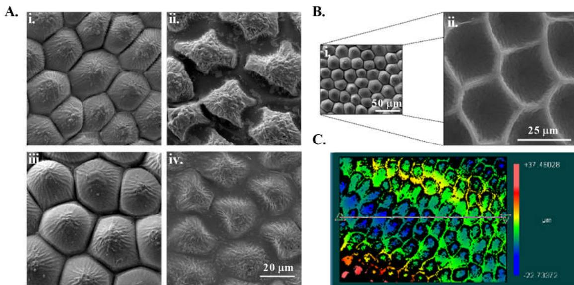
**Figure 3.** SEM images of rose petal patterns on PDMS surfaces; (A) positive replicas of (i) fresh and (ii) dry red rose, (iii) fresh and (iv) dry white rose petal patterns; (B) fresh white rose
