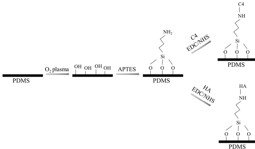
**Figure 2.** Functionalization of PDMS substrates with COL 4 and HA.
