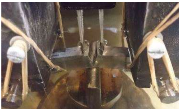
Fig. 4. Tested SENB specimen in an alcohol filled test rig on a tensile testing machine.
