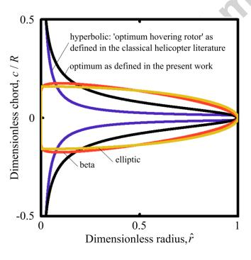
**Figure 1:** Comparison of the chord distribution for minimum total power for a revolving wing against a number of reference planforms. The so-called optimum distribution (black) is the chord distribution
