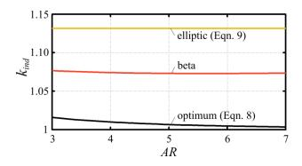
**Figure 3:** Variation of the induced power factor with wing aspect ratio. Wing twist is zero in each case. The value of  $k_{ind}$  is evaluated based on the method developed in reference [21].
