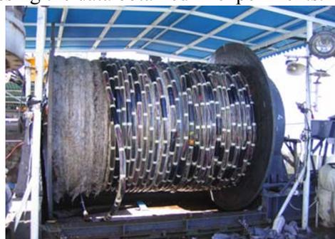
Fig. 17 Seismic streamer cable rolled on the wheel.
