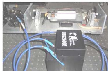
Fig. 11 YAG laser of LIBS.
