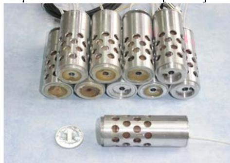
Fig. 14 Fiber seismic hydrophones.
