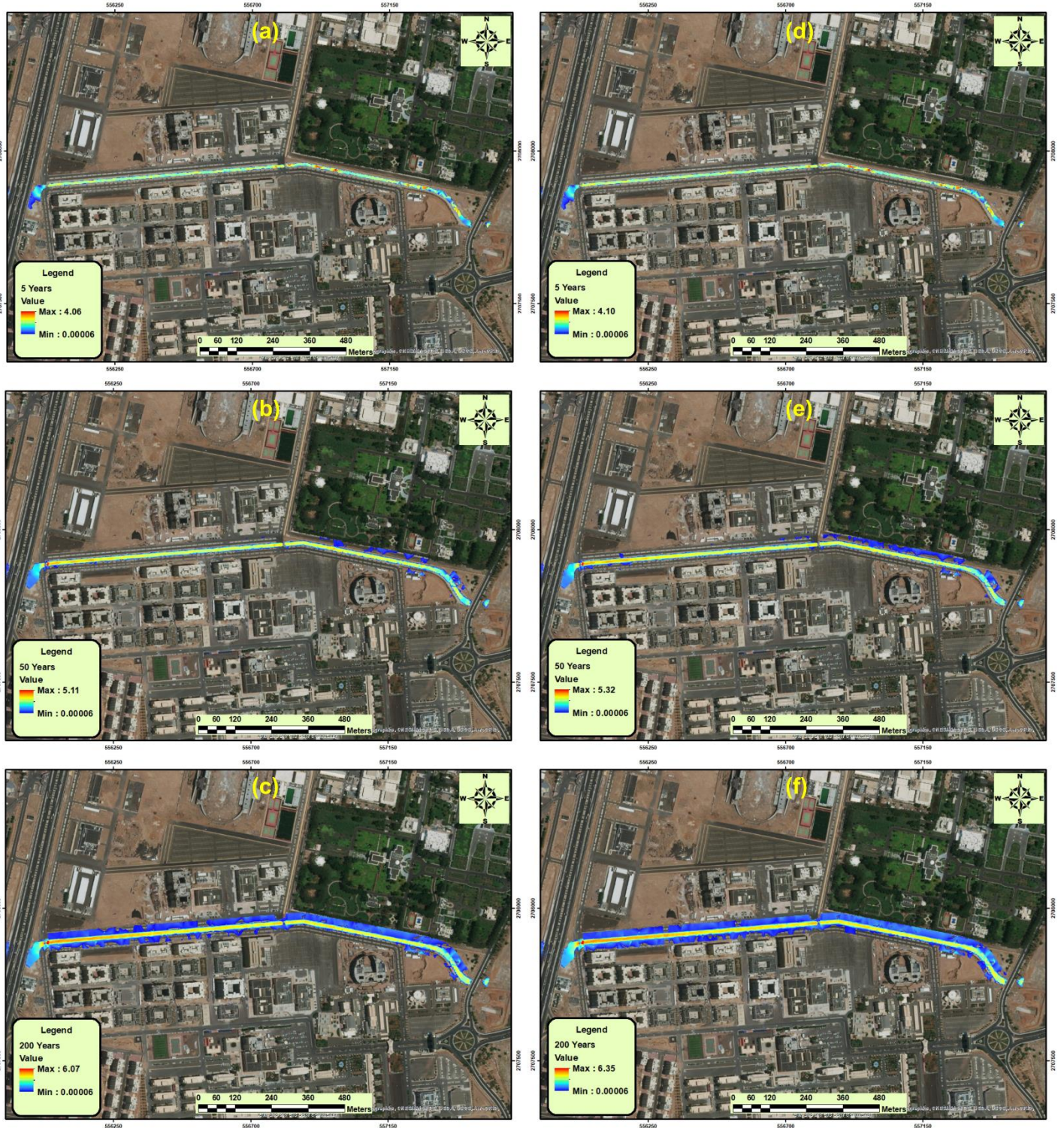
Figure 17 Flood inundation mapping of the Islamic University channel, where a, b, and c represent the return periods of 5, 50, and 200 years for the designed RDPs, and d, e, and f represent the return periods of 5, 50, and 200 years for the SCS type II RDPs, respectively
