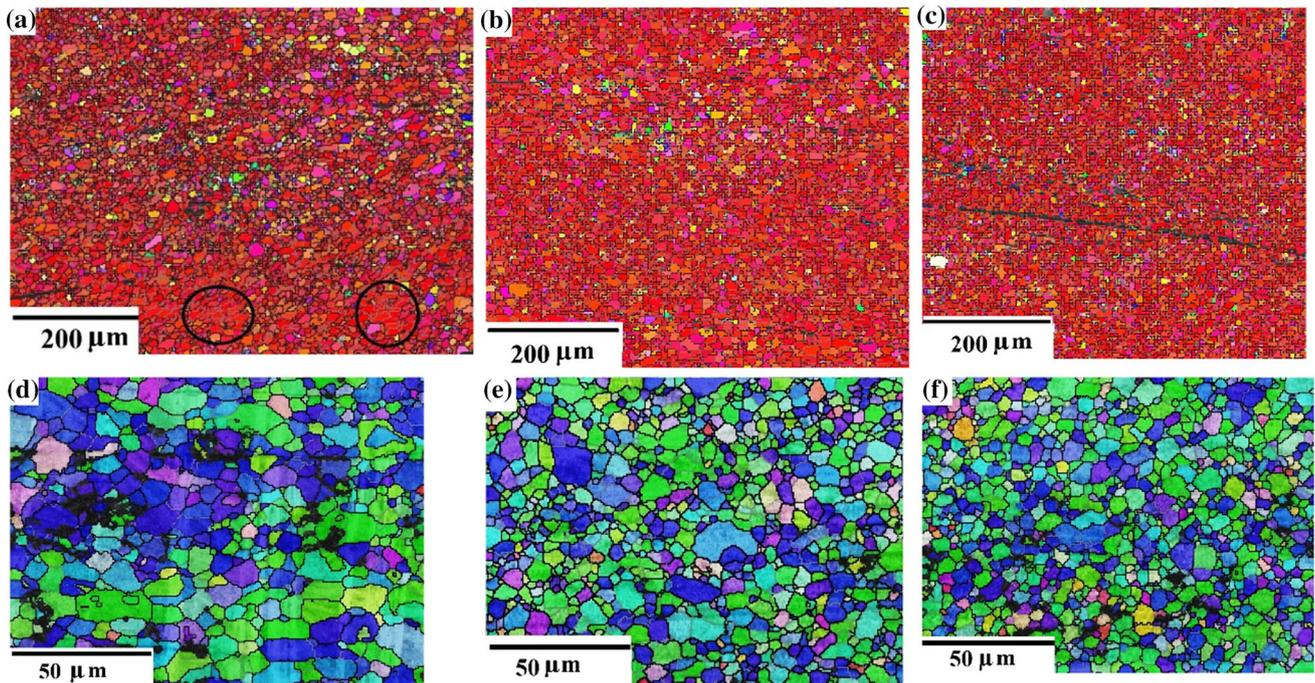
**Figure 5** EBSD images over the cross sections of an HPT-processed Mg sample after one turn. **a–c** Images from the top to the bottom, the view direction toward the upper surface. **d–f** High magnification images, the view direction toward the normal of the
