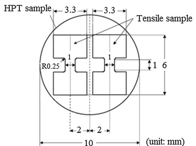
**Figure 1** Dimensions of mini-tensile samples cut from HPT disks [19].
