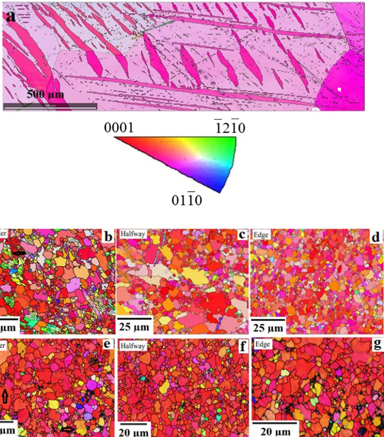
**Figure 2** EBSD images of the surface in **a** cast Mg and in HPT-processed Mg with **b–d** 1 and **e–g** 5 turns; the positions are **b**, **e** center, **c**, **f** halfway and **d**, **g** edge of the samples; high-angle
