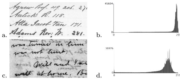
Fig. 4: Examples of global gray-level histograms: a relatively clean document (a), its corresponding gray-level histogram (b), an ancient degraded document (c) and (d) its corresponding histogram (more scattered and irregular than in b). The gray-level histogram is used to provide a first indication of the quality of the document.
