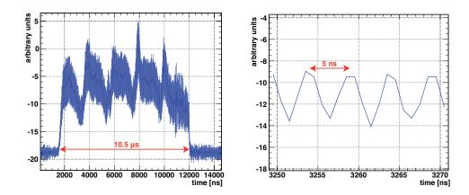
**Figure 4**. Example of a specially selected proton extraction waveform measured with the BCT detector BFCTI400344 to show the five-peak structure reflecting the proton losses in the PS Continuous Transfer extraction mechanism. This structure is more pronounced than for the majority of the waveforms. A blow-up of the waveform (right plot) shows that the 200 MHz SPS radiofrequency is resolved.
