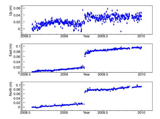
**Figure 7**. Monitoring of the PolaRx2e GPS antenna position at LNGS showing the slow earth crust drift and the fault displacement due to the 2009 earthquake in the L'Aquila region. Units for the horizontal (vertical) axis are years (metres).
