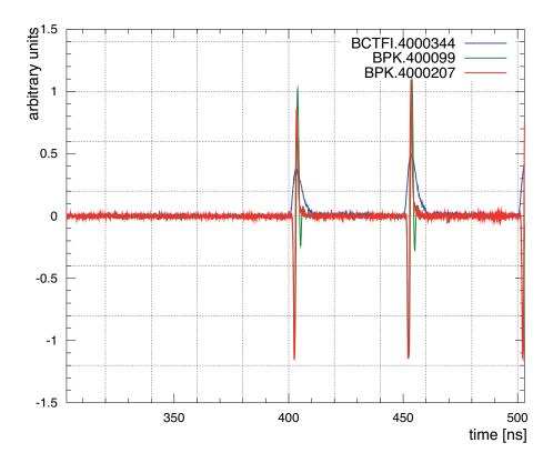
Figure 8. Comparison between the signals of the BCT and of the fast pick-up detectors after compensating for  $\Delta t_{\rm BCT}$ .
