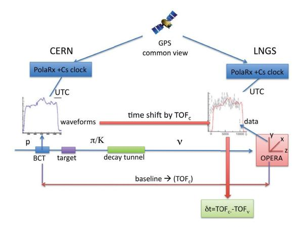
Figure 5. Schematic of the time of flight measurement.
