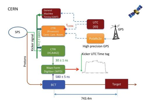
**Figure 3**. Schematic of the CERN SPS/CNGS timing system. Green boxes indicate detector time-response. Orange boxes refer to elements of the CNGS-OPERA synchronisation system. Details on the various elements are given in section 6.
