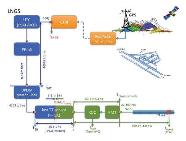
Figure 6. Schematic of the OPERA timing system at LNGS. Blue delays include elements of the time-stamp distribution; increasing delays decrease the value of  $\delta t$ . Green delays indicate detector time-response; increasing delays increase the value of  $\delta t$ . Orange boxes refer to elements of the CNGS-OPERA synchronisation system.
