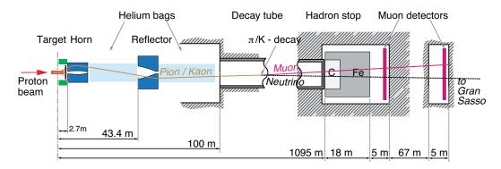
Figure 2. Layout of the CNGS beam line.
