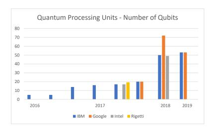
Fig. 1 Development in the number of qubits in published quantum processing units. However, it should be noted that development in coherence and other factors influencing computability are not reflected in this chart
