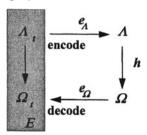
object (left) and to an object morphism (right). The morphisms  $e_A$  and  $e_Q$  representing the links to the environment are called *encoding* and *decoding* morphisms accordingly. The encoding morphism "translates" the commands of the environment into commands, which the process part of the object "understands", while the decoding one does the reverse. Should there be other behaviour morphisms with corresponding domains and encoding
