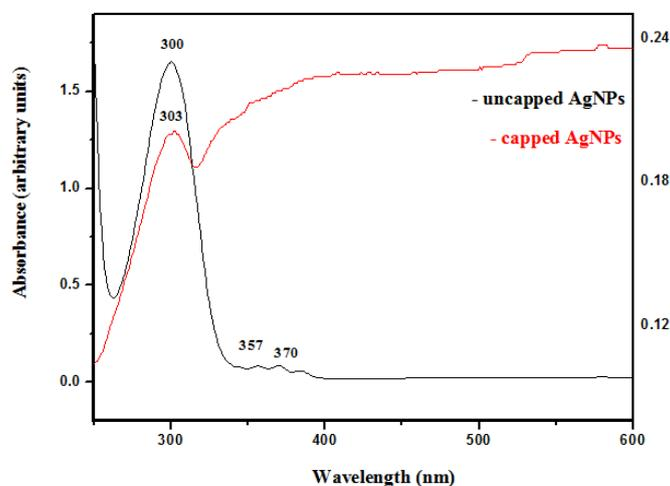
**Fig.3 UV-visible spectra of uncapped and capped silver nanoparticles**
