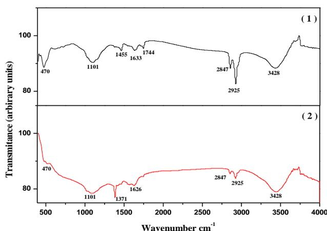
Fig.6 FTIR spectra of uncapped (1) and capped (2) silver nanoparticles.
