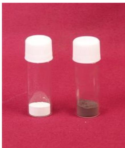
**Fig.1: Photographs of prepared uncapped and capped silver nanoparticles under room light.**
