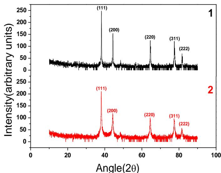
**Fig.4. X-Ray Diffraction pattern for powder samples of uncapped (1) and capped (2) silver nanoparticles**
