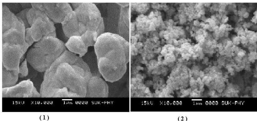
Fig.5 SEM images of uncapped (1) and capped (2) silver nanoparticles
