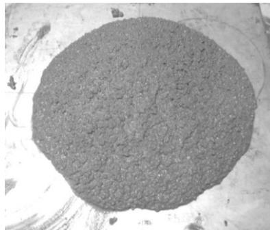
**Fig. 4.** slump flow- Mix#1
