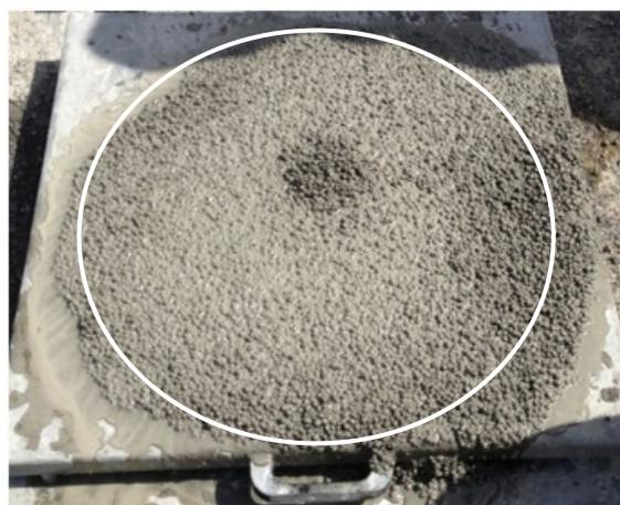
Fig. 8. slump flow – field application.
