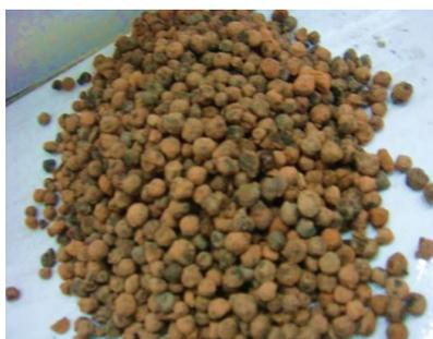
**Fig. 2.** sintered pulverized-fuel ash aggregates
