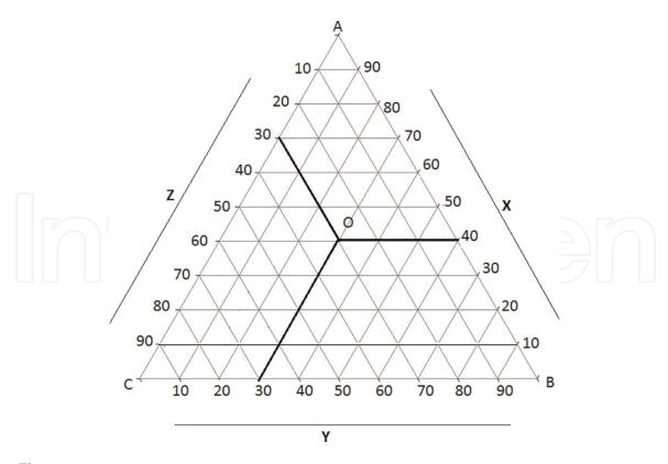
**Figure 1.**Typical ternary diagram indicating the composition of A, B, and C at point O.
