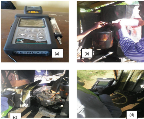
Figure 4. (a) KANE AUTOplus gas analyzer, (b) blended fuel being poured into the fuel tank of diesel engine, (c) gas emission analysis and (d) saving of analysis results on analyzer.
