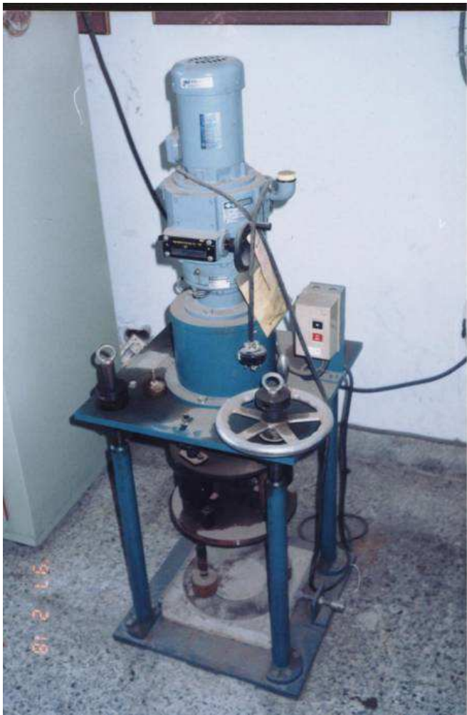
Fig. 2.3. Revolving disk abrasion test machine
