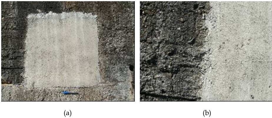
Fig. 11. Application point of repair material. (a) Reference concrete without additions. (b) Detail of the border between the RM and the substrate.
