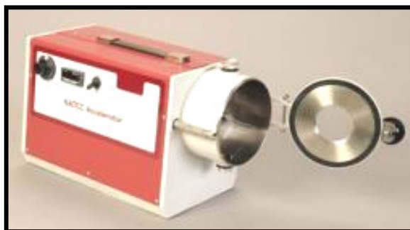
Fig. 8. Accelerator abrasion tester
