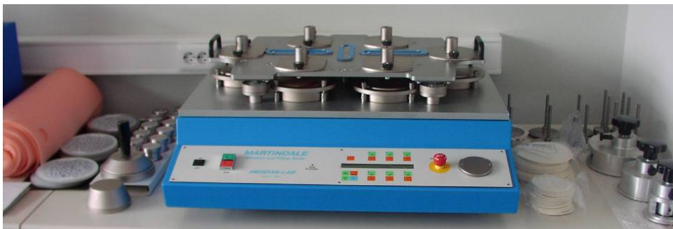
Fig. 1. Martindale abrasion testing apparatus
