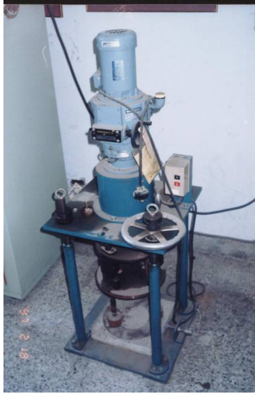
Fig. 2.3. Revolving disk abrasion test machine
