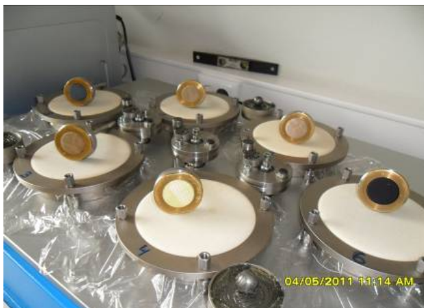
Fig. 6. Martindale abrasion tester prepared for wet abrasion
