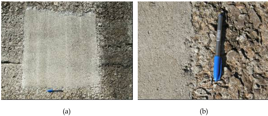
Fig. 12. Application point of repair material. (a) Concrete with addition of recycled LDPE in the content of 2.5%. (b) Detail of the border between the RM and the substrate.
