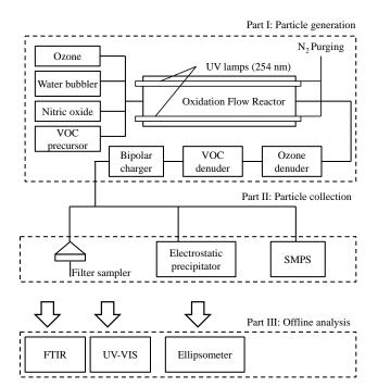
**Figure 1.** Schematic diagram of experimental apparatus. (I) Production of secondary organic material in aerosol form. (II) Sampling of particles onto a Teflon filter and growth of a thin film by electrostatic precipitation of particles onto a silicon substrate. (III) Fourier transform infrared spectroscopy (FTIR), ultraviolet–visible spectroscopy (UV–VIS), and spectroscopic ellipsometry of collected secondary organic material.
