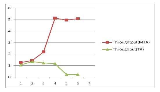
Fig 2 Throughput (Mbps/sec) Vs No of Faulty Nodes
