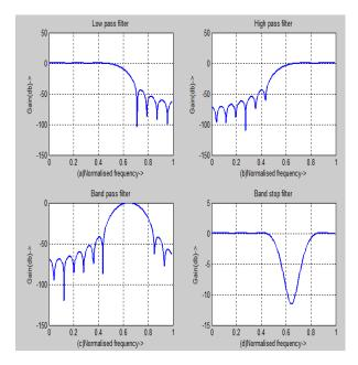
Fig.3: Filters using Hanning window (a) low pass (b) high pass (c) band pass (d) band stop
