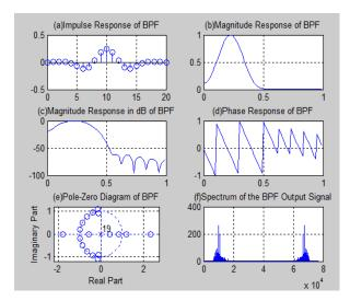
Fig.12: Speech signal analysis for band pass filter using Blackman window (order of filter=20)
