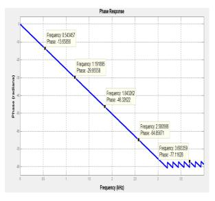
Fig.4: Phase response of Hanning window for low pass filter (N=64)
