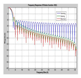
Fig.8: Frequency response of window function
