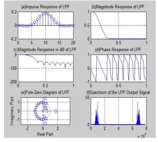
Fig.10: Speech signal analysis for low pass filter using hamming window (order of filter=20)
