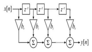
Fig.1: A discrete-time FIR filter of order N. The top part is an N-stage delay line with N + 1 taps.
