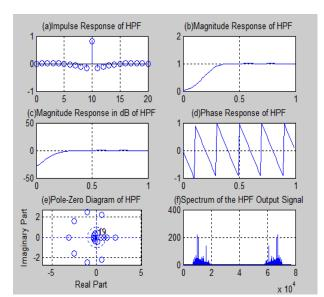
Fig.11: Speech signal analysis for high pass filter using Blackman window (order of filter=20)
