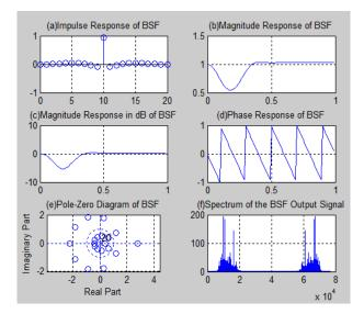
Fig.13: Speech signal analysis for Band stop filter using Hanning window (order of filter=20)
