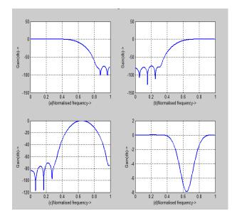
Fig.5: Filters using Blackman window (a) low pass (b) high pass (c) band pass (d) band stop
