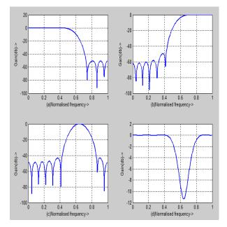
Fig.2: Filters using Hamming window (a) low pass (b) high pass (c) band pass (d) band stop
