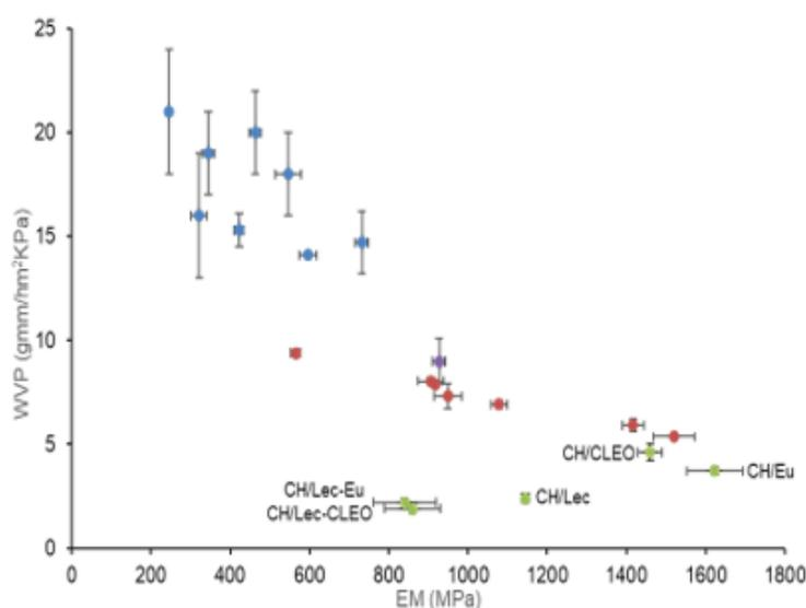
**Figure IV. 4** Water Vapor Permeability vs. Elastic Modulus of the films (● chapter 1, ● chapter 2, ● chapter 3/4, ● chapter 4).
