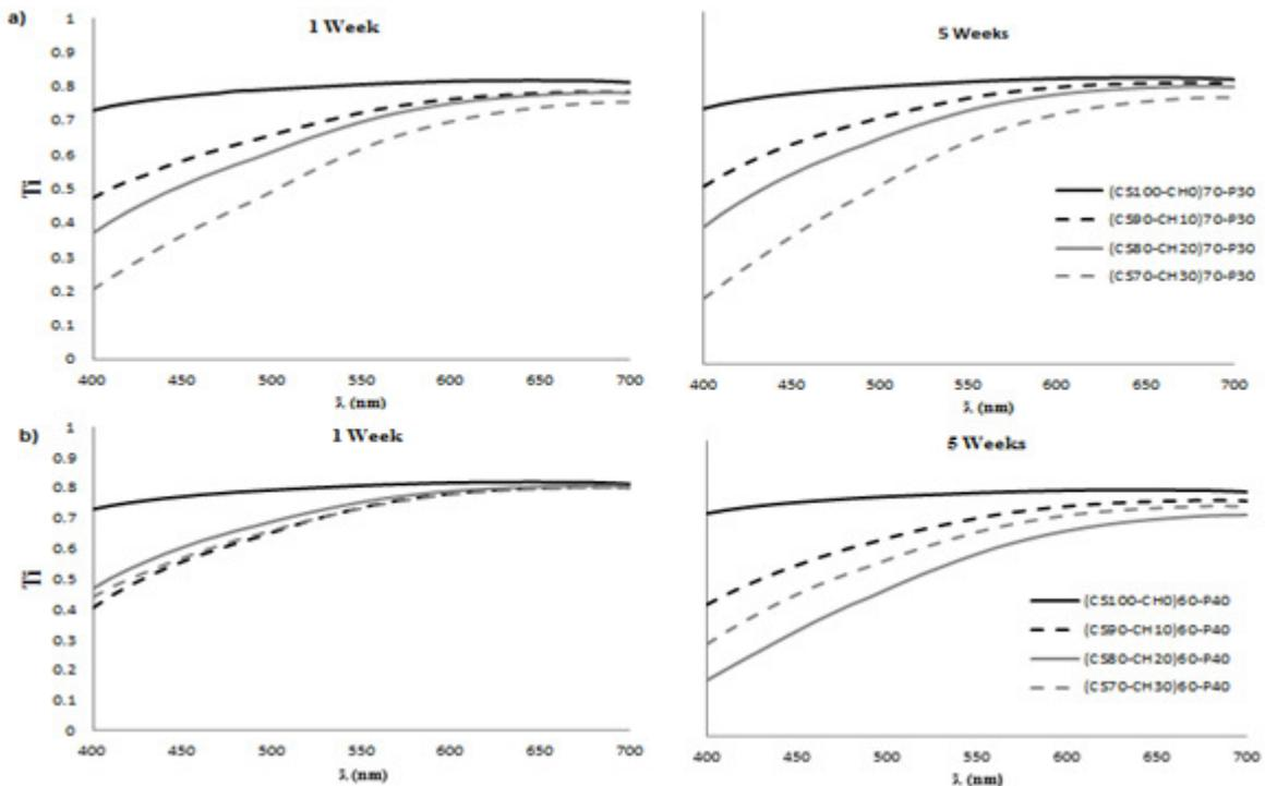
Figure 1.4. Spectral distribution of the internal transmittance ( $T_i$ ) of the films. (a) Ratio polymer: plasticizer 70:30. (b) Ratio polymer: plasticizer 60:40. After 1 week and 5 weeks of storage.
