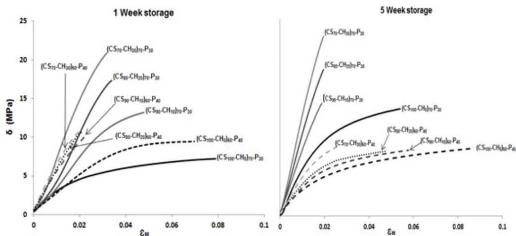
**Figure 1.3.** Typical stress-strain curves of the films after 1 week (left) and 5 weeks (right) of storage at 53 % RH.
