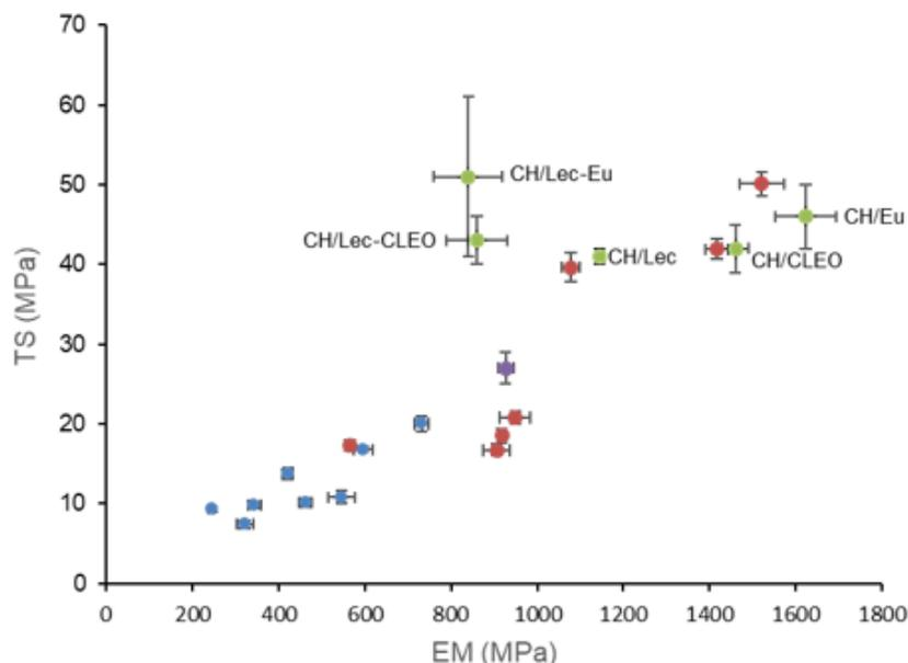
**Figure IV.1** Mechanical properties (Tensile Strength vs. Elastic Modulus) of the films (● chapter 1, ● chapter 2, ● chapter 3/4, ● chapter 5).
