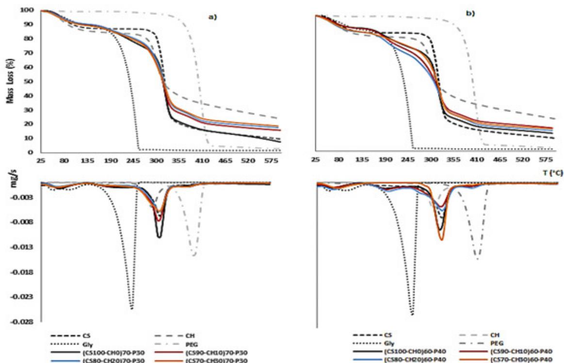
**Figure 1.2.** Typical thermogravimetric curves (mass loss vs. temperature) and first derivative (mg/s vs temperature) for **a)** Polymer: plasticizer proportion 70:30 and **b)** Polymer: plasticizer proportion 60:40.
