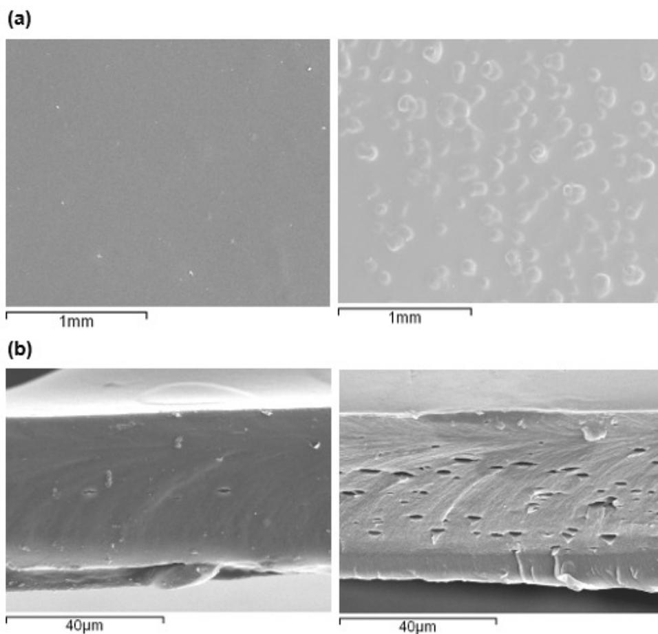
**Figure 5.3.** SEM micrographs of the (a) surface and (b) cross-section of chitosan film (left) and chitosan film with alginate-eugenol microcapsules (CH/M<sub>EU</sub>) (right).
