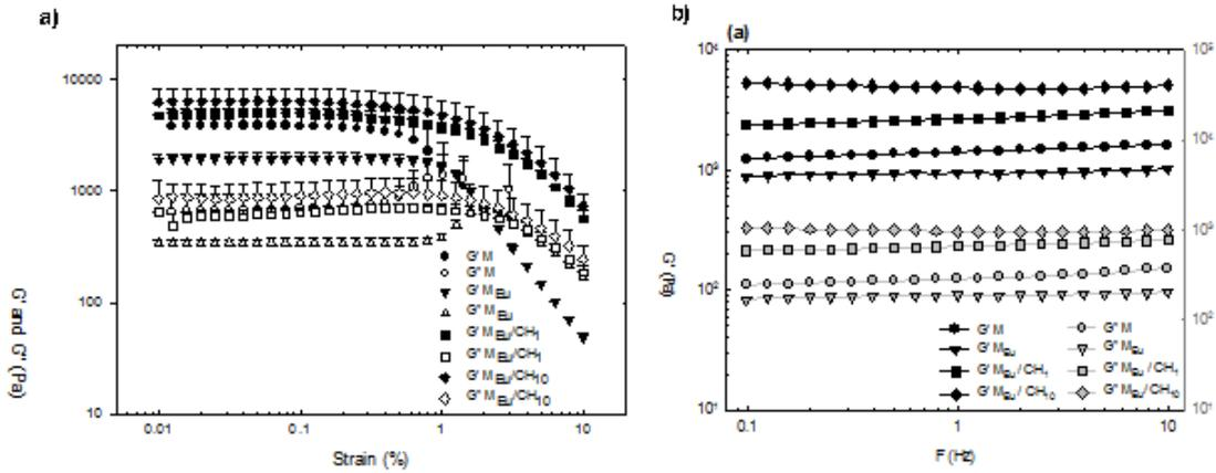
**Figure 5.2.** a) Strain sweep dependence of the storage moduli ( $G'$ ) and loss moduli ( $G''$ ) of the microspheres dispersions at 1 Hz and b) Frequency dependence of the storage moduli ( $G'$ ) and loss moduli ( $G''$ ).
