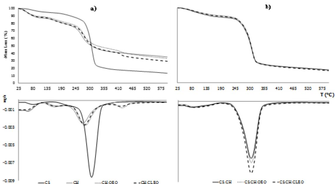
**Figure 2.2.** Typical thermogravimetric curves (weight loss vs. temperature) and first derivative (mg/s vs temperature) for a) monolayer films and b) bilayer films.
