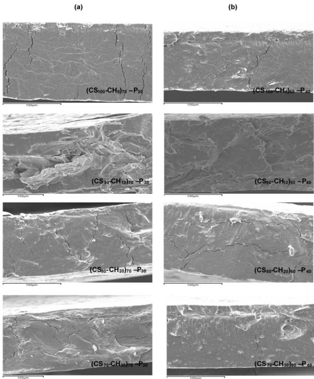
**Figure 1.1.** Scanning electron microscopy micrographs of the cross-sections of the films. **(a)** Polymer: plasticizer proportion 70:30. **(b)** Polymer: plasticizer proportion 60:40.
