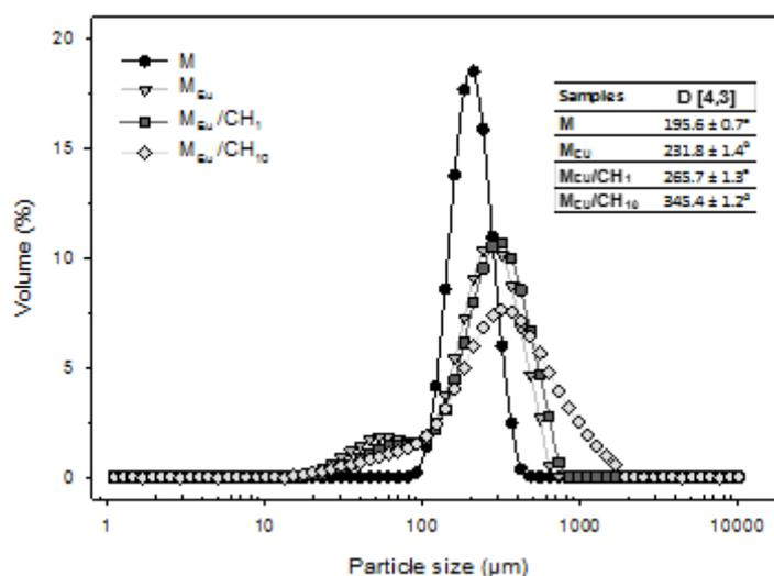
**Figure 5.1.** Typical particle size distribution curves of the microspheres.
