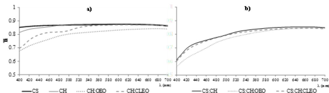
**Figure 2.3.** Spectral distribution curves of internal transmittance ( $T_i$ ) of the (a) monolayer and (b) bilayer films.
