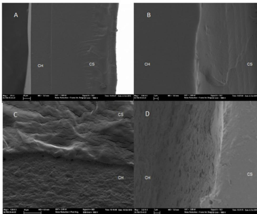
**Figure 2.1.** FESEM micrographs of cross-sections of bilayer films A and B) CS-CH at different magnifications C) CS-CH-OEO showing the layer interface, D) CS-CH-CLEO showing the layer interface.
