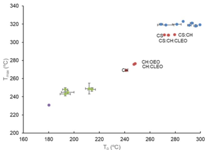
**Figure IV.6**  $T_{max}$  versus  $T_0$ , obtained from thermogravimetric analyses of all the films (● chapter 1, ● chapter 2, ● chapter 3/4, ● chapter 4).
