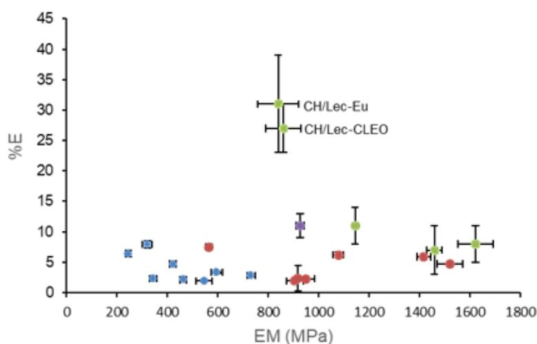
**Figure IV.2** Mechanical properties (stretchability vs. Elastic Modulus) of the films (● chapter 1, ● chapter 2, ● chapter 3/4, ● chapter 5).
