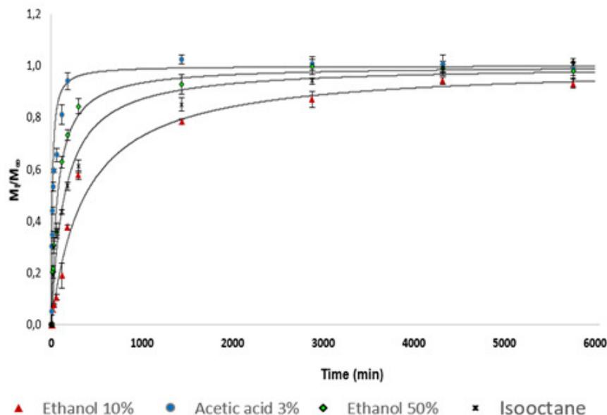
**Figure 5.5.** Eugenol release curves from chitosan films containing encapsulated eugenol-alginate microcapsules in the food simulants: ethanol 10 % (v / v), ethanol 50 % (v / v), acetic acid 3 % (w / v) and Isooctane. Experimental data (symbols) and Fitted Peleg's (continuous lines).
