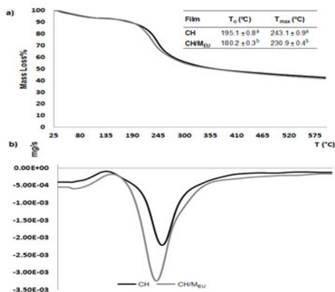
**Figure 5.4.** a) Typical thermogravimetric curves (mass loss vs. temperature) and b) first derivative (mg/s vs. temperature) for CH and CH/M<sub>EU</sub> films.
