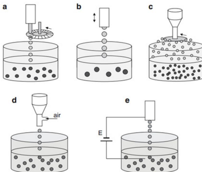
**Figure I.7** Set-ups of different ways of making alginate microspheres by extrusion. Aqueous solution alginate and active are atomized by jet-cutter (a), pipette or vibrating nozzle (b), atomizing disk (c), coaxial air-flow (d), or electrostatic potential (e). The droplets fall into a batch of  $\text{Ca}^{2+}$ , resulting in instantaneous formation of calcium alginate microspheres (Zuidam & Nedovic, 2010).
