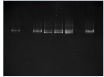
*Plate 4: 20%:80% DGGE fingerprints of PCR- amplified region using GCV3F and V3R of 16S rDNA from effluent bacterial communities. Lanes:1-3,effluent samples from river; 4-6 effluent from clarifier, and 7and 8samples from retention pond gate.*
