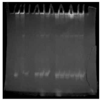
*Plate 5: 30%: 50% DGGE fingerprints of PCR- amplified region using GCV6 –V8F and V6-V8R of 16S rDNA from effluent bacterial communities. Lanes: 1-3, effluent samples from clarifier; 4-6samples from river; 7-9, samples from processed water and lanes 10-12, samples from retention pond gate.*
