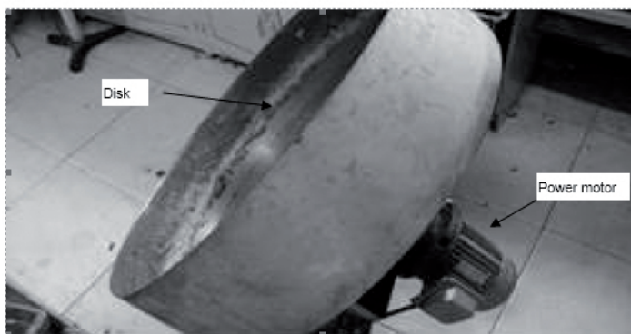
Figure 1. Disk granulator used to make the newly developed fertilizer.
