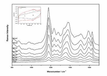
Figure 5: Raman spectra of polyaniline at a different potential; insert: CV curve recorded for the polyaniline film Please click here to view a larger version of this figure.
