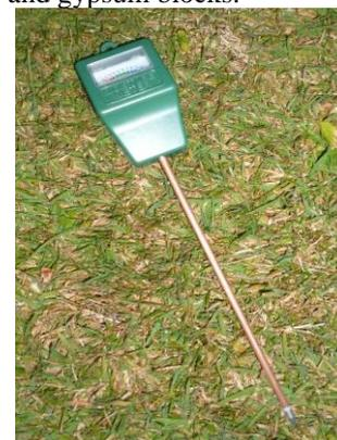
**Fig.7. Soil Moisture Sensor**
