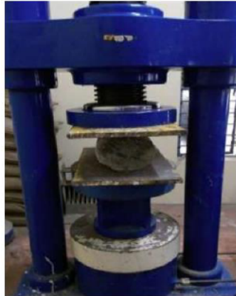
Figure 6 Split Tensile strength setup used in our investigation
