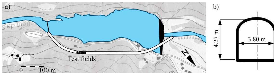
**Figure 3.** (a) Overview and (b) cross section of the Runcahez SBT (position  $46^{\circ}40'45.0''$  N  $8^{\circ}58'05.7''$  E; adapted from [18]).
