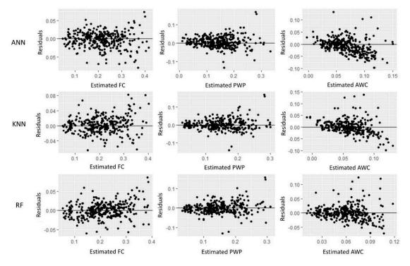
**Figure 7.** Residuals of field capacity (FC), permanent wilting point (PWP), and available water content (AWC) estimations using different machine learning algorithms.
