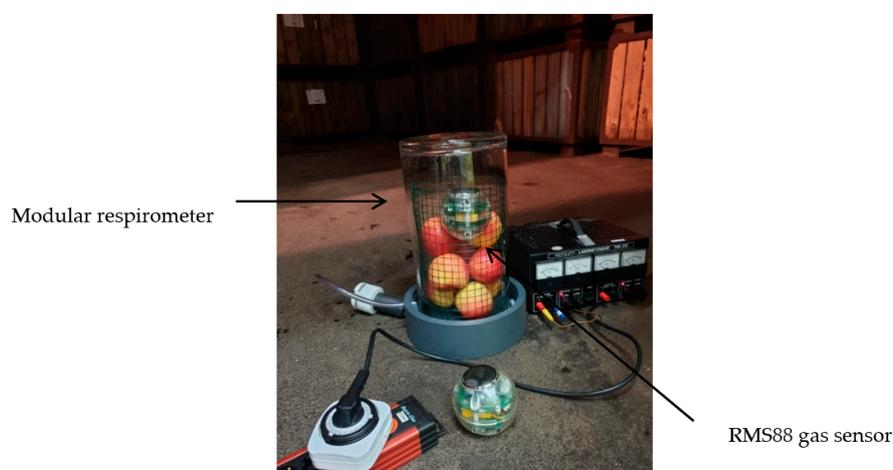
**Figure 2.** The modular respirometer filled with Pinova apples along with the RMS88 gas sensor installed inside a commercial CA storage unit at 2% O<sub>2</sub>, 1.3% CO<sub>2</sub> and 2 °C.
