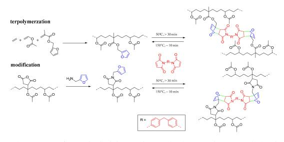
**Scheme 1.** Furan-functionalized ethylene–vinyl acetate (EVA) via terpolymerization (**top**) and post-polymerization modification (**bottom**) and subsequent thermoreversible cross-linking with bismaleimide via (retro) Diels–Alder (DA) chemistry.
