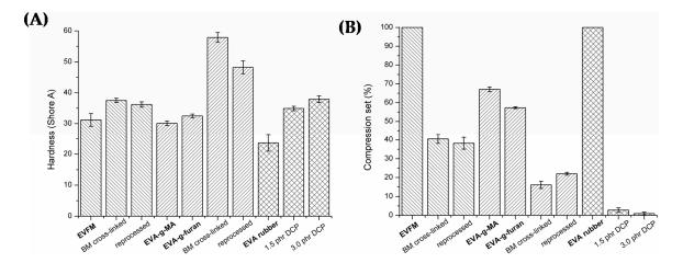
**Figure 3.** (A) Hardness and (B) compression set at room temperature of EVFM, EVA-g-MA, EVA-g-furan, and EVA rubber precursors and their BM/DCP cross-linked and reprocessed products. The error bars indicate  $\pm$  1 standard deviation.
