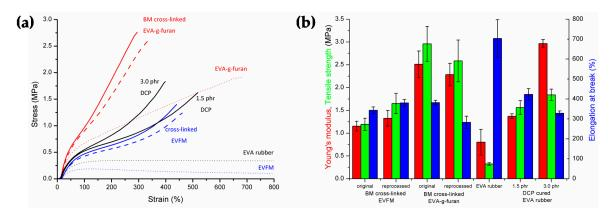
**Figure 4.** (a) Median stress–strain curves of non-cross-linked (dashed lines), BM/peroxide cross-linked (bold lines), and reprocessed (normal lines) EVA-*g*-furan, EVFM, and EVA rubber samples and (b) the average values for the Young's modulus, tensile strength, and elongation.
