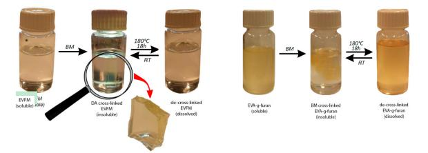
**Figure 1.** Solubility in 1,2,4-trichlorobenzene at room temperature of non-cross-linked, BM cross-linked, and de-cross-linked samples of EVFM (**left**) and EVA-*g*-furan (**right**).
