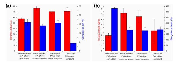
**Figure 6.** (a) Hardness and compression set at room temperature and (b) tensile strength and elongation at break of BM cross-linked EVA-*g*-furan gum rubber and compounds, reprocessed compounds, and DCP-cured EVA rubber compounds. The error bars indicate  $\pm 1$  standard deviation.
